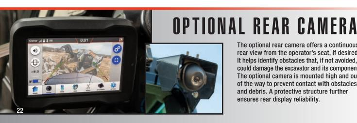
The optional rear camera offers a continuous rear view from the operator's seat, if desired. It helps identify obstacles that, if not avoided, could damage the excavator and its components. The optional camera is mounted high and out of the way to prevent contact with obstacles and debris. A protective structure further ensures rear display reliability.
