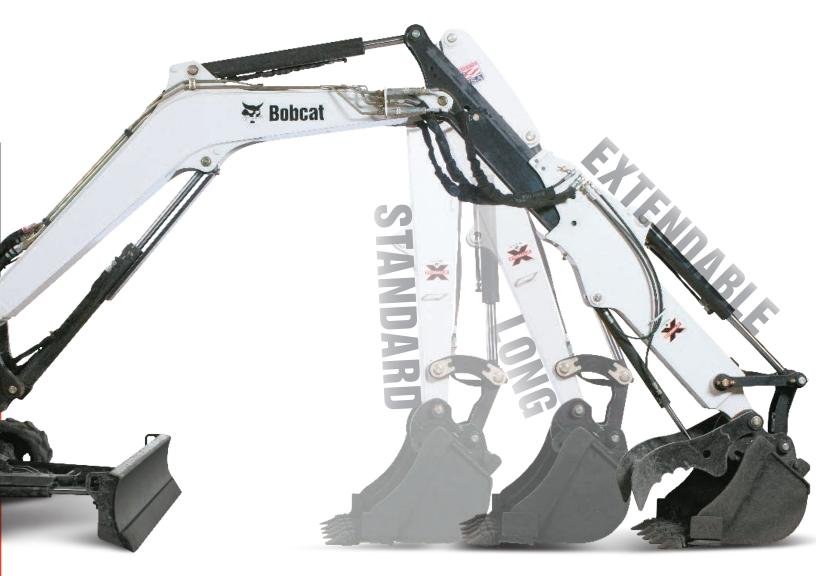
Bobcat compact excavators provide you with the choice of three different lift arm configurations. This allows you to customize the excavator's breakout forces and reach to the work you do most often. Choose a standard arm, long arm or extendable arm.
