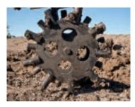
The open rim sheep-foot design utilizes the weight of the wheel and down pressure from the carrier to achieve compaction, without the need for auxiliary hydraulics.
