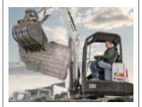
Use the handy hydraulic clamp to move broken concrete, tree stumps and other odd-shaped objects. Use with trenching bucket or 3-tine grapple.
