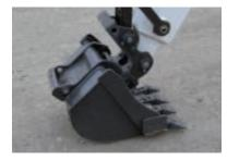
3. Retract attachment cylinder completely. Lower attachment to ground. Disengage X-Change pins from attachment ears using boom and arm functions.
