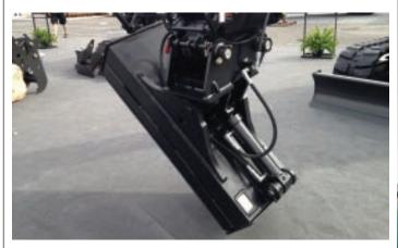
Gives the operator flexibility to shape holes and ditches by tilting the bucket left or right 40°. Smooth lip for finished surface.
