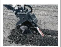
Tackle trenching jobs with the costeffective Bobcat excavator and trencher. With a 2-foot dig depth, it's ideal for light-to-medium trenching jobs. The versatile X-Change mount is standard.
