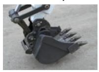
2. Using the attachment function, curl the X-Change forward until it has full contact with the back of the attachment. Lower boom to the ground until the X-Change is fully seated in the attachment interface.
