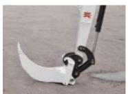
The frost and rock ripper is used to penetrate and scarify frost and hard ground.
