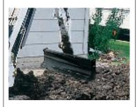
Great attachment for finish grading, backfilling and leveling. Combine with a Hydra-Tilt or PowerTilt™ attachment to create slopes, grade and contour with ease.
