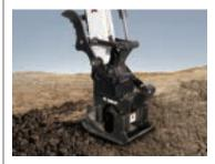
Choose from two models for quick, efficient trench compacting. Reduces the need for a man in the trench with a hand-operated compactor.
