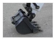
1. Fully retract attachment cylinder and align X-Change. Using the boom and arm functions, engage X-Change pins with attachment ears. Raise attachment slightly off ground using the boom function.
