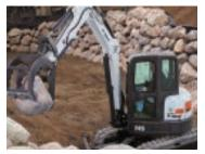
This tool makes easy work of handling bulky material such as brush, logs and landscaping stones. (Two sizes available.)
