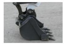
3. Insert attachment retaining pin completely through the X-Change and attachment. Install ring-lock pin.
