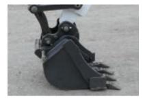
1. Place attachment on level ground surface. Remove ring-lock pin. Remove attachment
