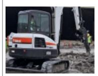
As many as four different hydraulic breakers, depending on excavator model, deliver from 60 to 1000 foot-pounds of impact energy for demolition projects.
