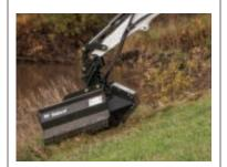
Expand the versatility of your compact excavator. Cut down brush, thick weeds and grass, even small trees with the Bobcat flail mower. It cuts aggressively and efficiently, with a direct-drive hydraulic motor that provides the optimum balance between torque and RPM, and tripleknife flails that rip through hard and soft woods, vines, grass and brush.
