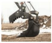
The Pro Clamp™ System adds incredible versatility with interchangeable tools that adjust to the task. Just attach the Pro Clamp base. Pin on the adjustable material clamp to grab. Switch to the reversible grading tool to grade. And if you need more curling ability for loading trucks or extra visibility when trenching and digging around utilities, simply remove the tool and tuck the Pro Clamp base out of the way.
